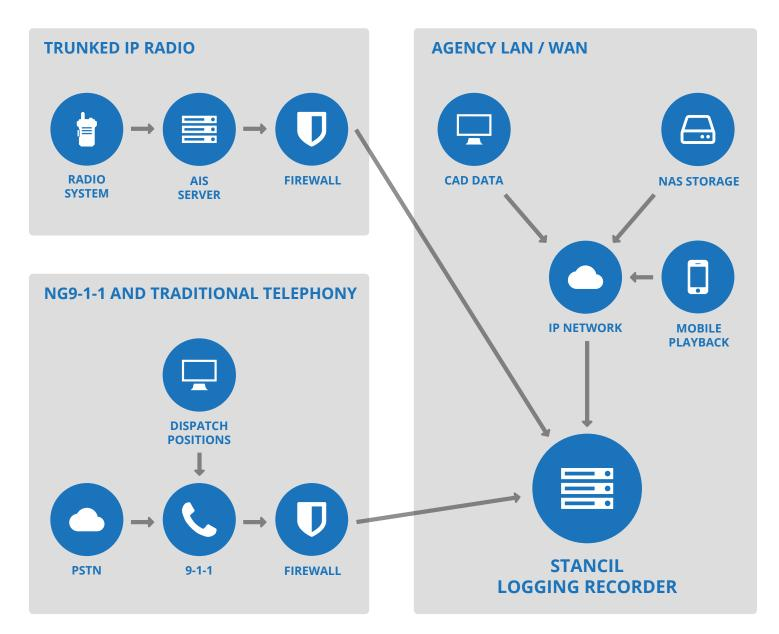
SUPPORTS ENCRYPTED AND NON-ENCRYPTED P25 IP RADIO RECORDING INCLUDING CAPTURE OF ALL TALK GROUP NAMES, SUBSCRIBER ID AND ALIAS
