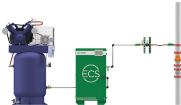
Sprinkler System with Nitrogen Generator (Vent placed at furthest point on the system)
